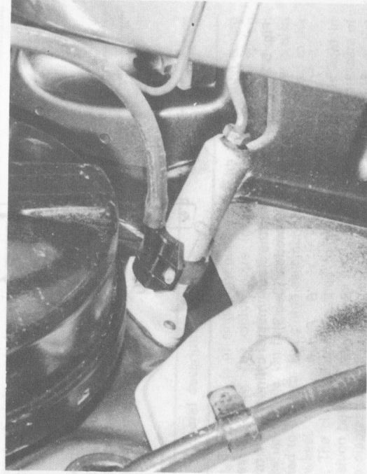
3.5 View of the clutch master cylinder from the engine compartment on RHD 900 models
